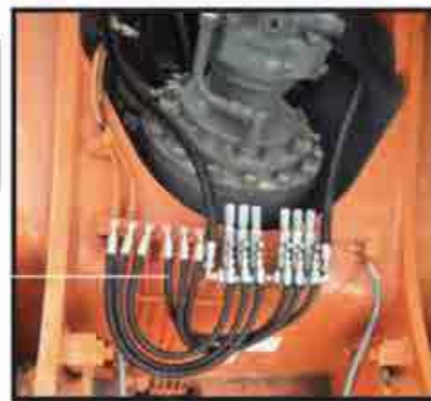
Hartex Hydraulic Grease Pump installation on EX-1200
