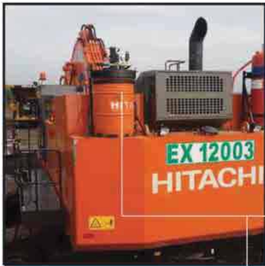
Hartex Hydraulic Grease Pump installation on EX-1200
